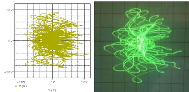
Fig. 11.  $y$ - $w$  phase portrait results of the electronic circuit of the new hyperchaotic system obtained from Orcad-PSpice and the oscilloscope screen respectively.
