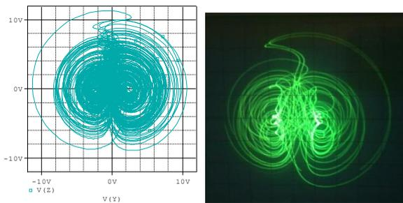
Fig. 8.  $y$ - $z$  phase portrait results of the electronic circuit of the new hyperchaotic system obtained from Orcad-PSpice and the oscilloscope screen respectively.
