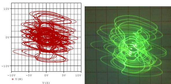
Fig. 9.  $x$ - $w$  phase portrait results of the electronic circuit of the new hyperchaotic system obtained from Orcad-PSpice and the oscilloscope screen respectively.
