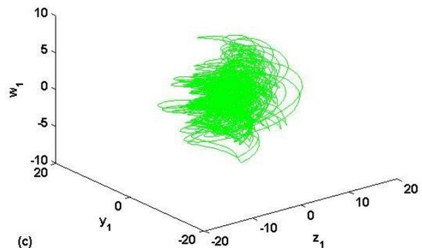
Fig. 2. Hyperchaotic attractors of the system (2.2) with no equilibria for the case  $(a, b, c, k, m) = (5, 5, 0, 1, 1)$  with initial conditions  $(5, -0.1, 1, 2)$ : (a) attractor projected in 3-D space  $x_1 - y_1 - z_1$ ; (b) attractor projected in 3-D space  $x_1 - z_1 - w_1$ ; (c) attractor projected in 3-D space  $y_1 - z_1 - w_1$ .
