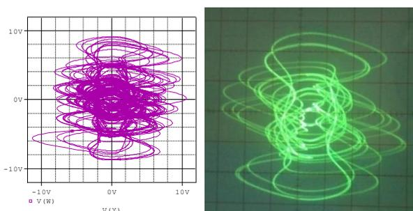
Fig. 10.  $y$ - $w$  phase portrait results of the electronic circuit of the new hyperchaotic system obtained from Orcad-PSpice and the oscilloscope screen respectively.
