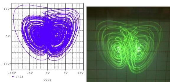
Fig. 7.  $x$ - $z$  phase portrait results of the electronic circuit of the new hyperchaotic system obtained from Orcad-PSpice and the oscilloscope screen respectively.
