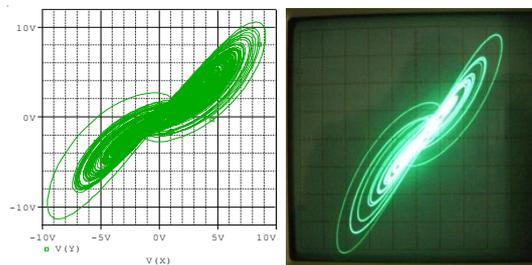
Fig. 6.  $x$ - $y$  phase portrait results of the electronic circuit of the new hyperchaotic system obtained from Orcad-PSpice and the oscilloscope screen respectively.
