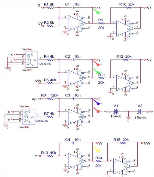
Fig. 5. The designed electronic circuit schematic of the new hyperchaotic system(2.2).
