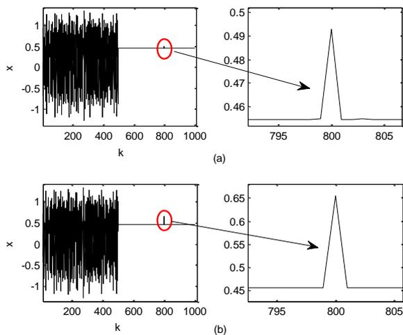
Fig. 7. Stabilization performance under an external disturbance applied (a) proposed method (b) backstepping method.
