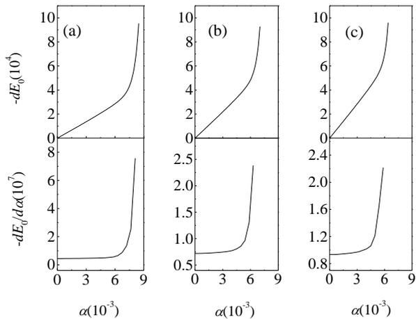
Fig. 2. Ground-state energies and their numerical derivatives of the acoustic polarons in a free-standing quantum well with the  $L = 0.3$ , as functions of the e-p coupling constant  $\alpha$  for (a)  $q_0 = 150$ , (b)  $q_0 = 180$  and (c)  $q_0 = 200$ , respectively.
