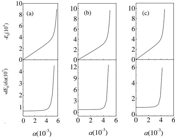
Fig. 1. Ground-state energies and their numerical derivatives of the acoustic polarons in a free-standing quantum well with the  $L = 0.03$ , as functions of the e-p coupling constant  $\alpha$  for (a)  $q_0 = 150$ , (b)  $q_0 = 180$  and (c)  $q_0 = 200$ , respectively.
