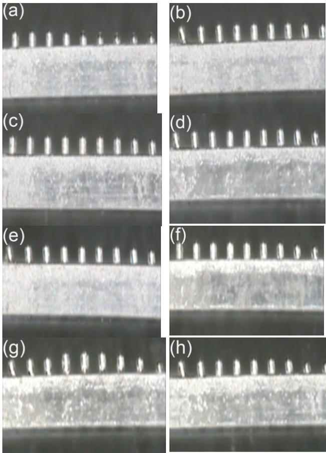
Fig. 9. Digital images of microlenses with different injection times. (a).  $t=0.4s$ ,  $W=73.15mg$ . (b).  $t=0.6s$ ,  $W=73.58mg$ . (c).  $t=0.8s$ ,  $W=73.72mg$ . (d).  $t=1.0s$ ,  $W=73.62mg$ . (e).  $t=1.2s$ ,  $W=73.55mg$ . (f).  $t=1.4s$ ,  $W=73.46mg$ . (g).  $t=1.6s$ ,  $W=73.32mg$ . (h).  $t=1.8s$ ,  $W=73.30mg$ .
