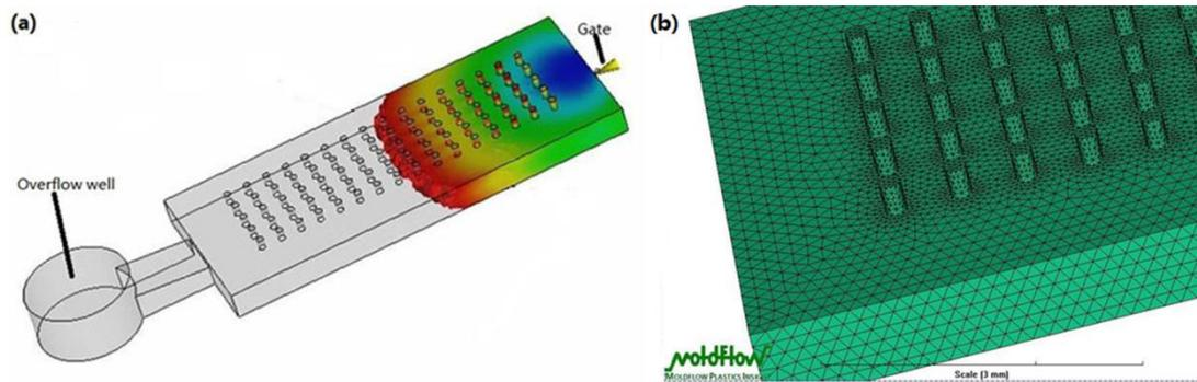
Fig. 7. 3D geometrical simulation model in MPI® software. (a). Overall model. (b). Detailed meshes.
