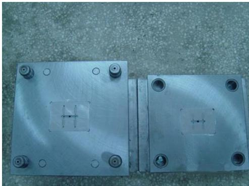
Fig. 5. Injection mold for the designed microlens array.
