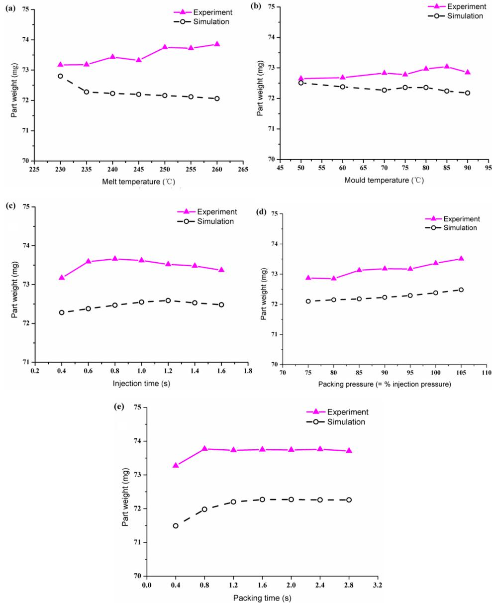
Fig. 8. Effects of processing parameters on the part weight of injection-molded microlens arrays from both the experimental and the simulation results.
