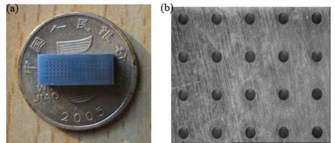
Fig. 3. Fabricated mold insert of micro column array using the modified LIGA process. (a) Nickel Mold insert. (b) Microscope image of microlenses with a diameter of 0.2 mm
