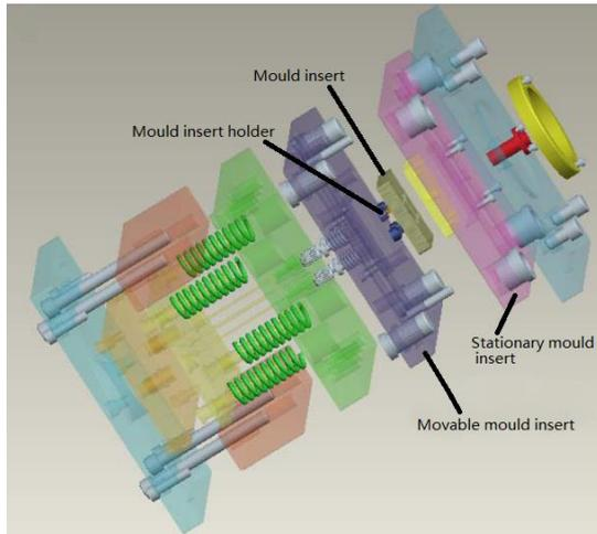
Fig. 4. 3D explosion drawing for the injection mold.
