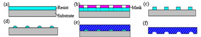
Fig. 2. Processing steps for the fabrication of mold insert with modified LIGA process. (a) Coating. (b) Exposure. (c) Develop. (d) Reflow. (e) Electroforming. (f) Molding.
