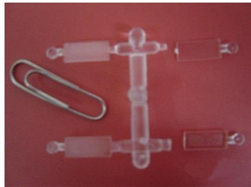
Fig. 6. Injection-molded microlens array with its runner system.
