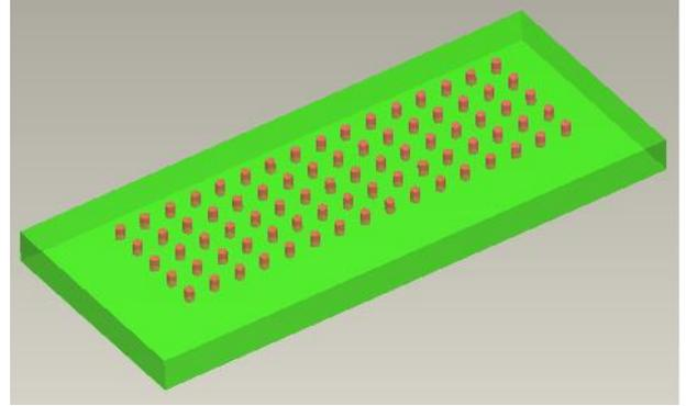
Fig. 1. Structure of designed microlens array.
