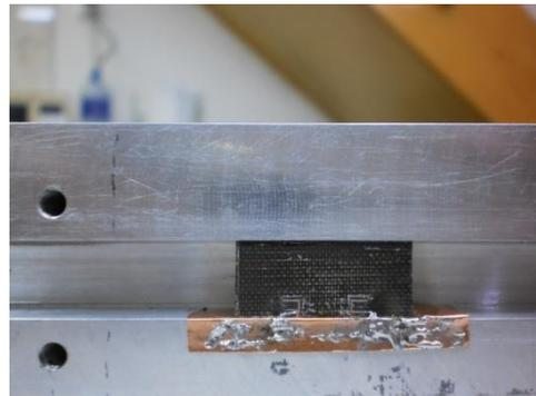
Fig. 15. Photograph of the fabricated printed-circuit insert, with two QWRs, placed in the  $E$ -plane of the waveguide.
