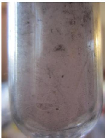
Fig. 3. The no-cracking  $\text{LaBr}_3:\text{Nd}^{3+}$  single crystal grown by vertical Bridgman process. The inner diameter of quartz crucible is 25 mm.
