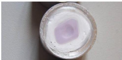
Fig. 4.  $\text{LaBr}_3:2.5\% \text{Nd}^{3+}$  Crystal ready for scintillation experiments is covered with Teflon tape and packaged by Al shell and quartz glass. The inner diameter of Al shell is 17 mm.
