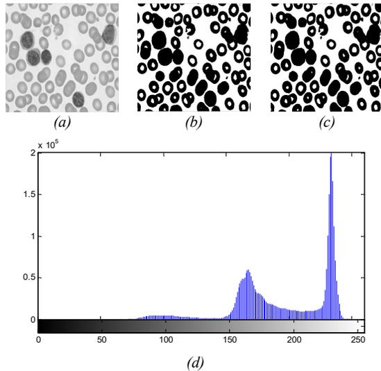
Fig. 5. a) K5 original image, b) Thresholded image by using Otsu method, c) Thresholded image by using TAHS method, d) Histogram of K5 image
