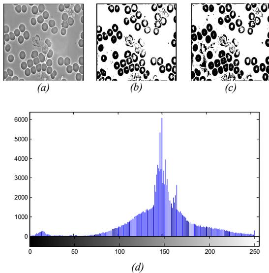
Fig. 6. a) K6 original image, b) Thresholded image by using Otsu method, c) Thresholded image by using TAHS method, d) Histogram of K6 image
