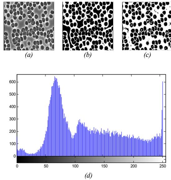
Fig. 4. a) K4 original image, b) Thresholded image by using Otsu method, b) Thresholded image by using TAHS method, d) Histogram of K4 image
