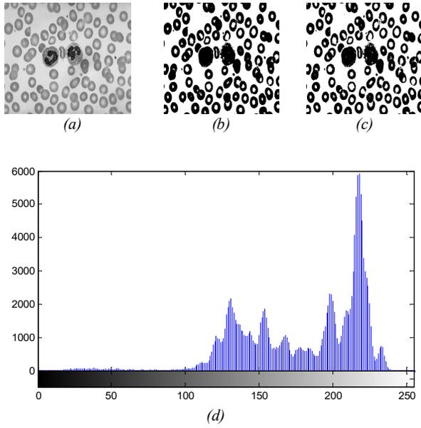
Fig. 1. a) Original image, b) Thresholded image by using Otsu method, b) Thresholded image by using TAHS method, d) Histogram of original image
