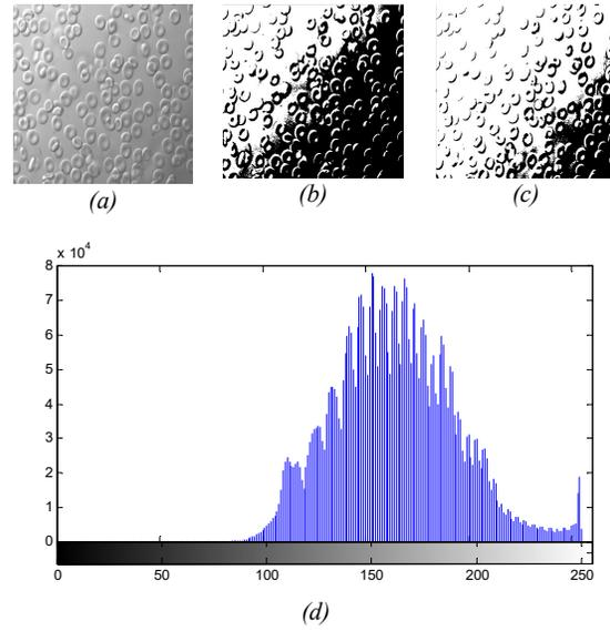
Fig. 3. a) K3 original image, b) Thresholded image by using Otsu method, b) Thresholded image by using TAHS method, d) Histogram of K3 image
