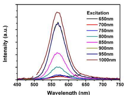
Fig. 7. Upconversion fluorescence spectra of WPU/silica/CdTe nanocomposites.
