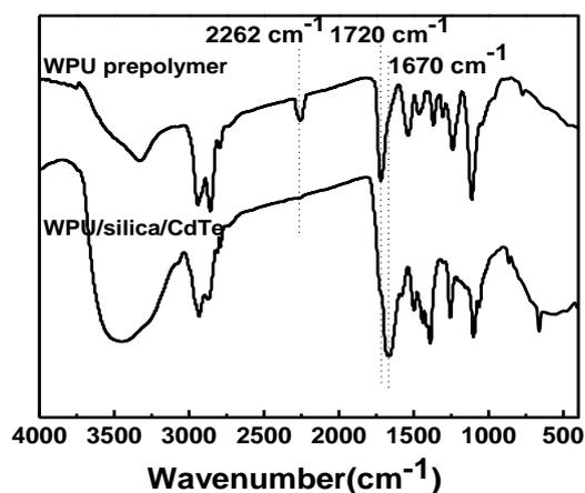
Fig. 3. FT-IR spectra of WPU prepolymer and WPU/silica/CdTe.
