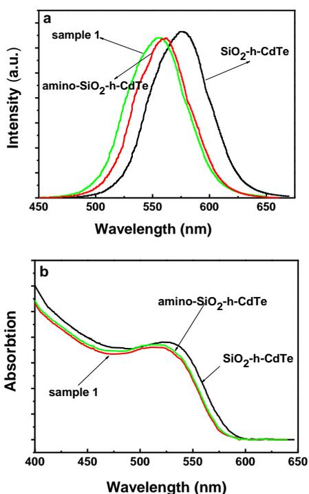
Fig. 6. PL and UV-vis absorption spectra of SiO<sub>2</sub>/CdTe, amino-SiO<sub>2</sub>/CdTe, Sample 1.
