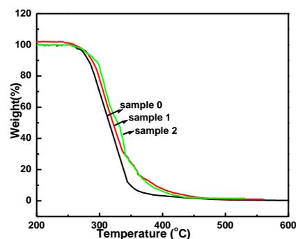
Fig. 5. TGA analysis of WPU/silica/CdTe.
