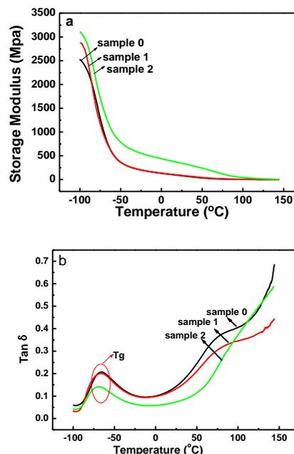
Fig. 8. Storage modulus (a) and  $\tan\delta$  (b) of WPU/silica/CdTe nanocomposites versus temperature.
