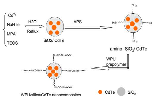
Fig. 1. Preparation of WPU/silica/CdTe nanocomposites.
