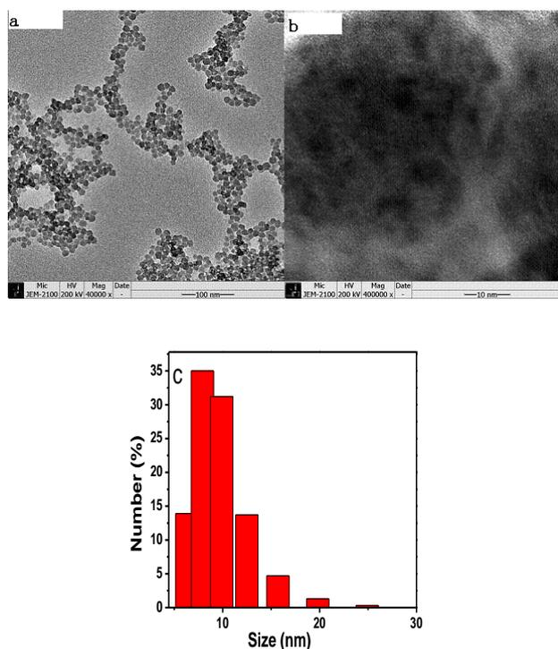
Fig. 4. Images of  $\text{SiO}_2$ -h-CdTe: (a) and (b) TEM image; (c) size distribution.
