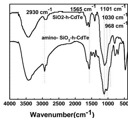
Fig. 2. FT-IR spectra of  $\text{SiO}_2$ -h-CdTe and amino- $\text{SiO}_2$ -h-CdTe.
