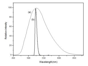
Fig. 3. Normalized 3PA induced up-convertion fluorescence (a) and lasing (b) spectra in PMMA with doped concentration of  $1 \times 10^{-2}$  mol/L
