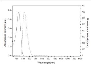
Fig. 2. Normalized one-photon absorption spectrum(solid line) and fluorescence spectrum(dot line) of TCFVTPA in chloroform at 1×10<sup>-5</sup> mol/L
